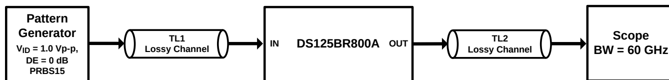
Figure 23. Test Setup Connections Diagram
